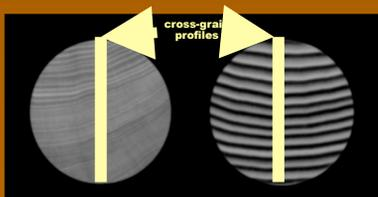
**Maple grain structure is more uniform than ash,** likely affecting several important mechanical properties. Profiles of CT data taken across the grain shows that the high density bands in ash and maple are nearly the same, but the intervening wood is much lower density in ash than in maple.
