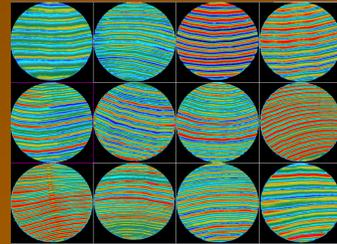
**Maple is denser than ash.** CT data can be interpreted directly in density units. Three maple bats were 10 – 15% denser than three corresponding ash bats. We found little variation along the length of the bats. For a given bat length and weight, the maple bats are thus slightly smaller in barrel diameter.
