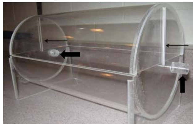
FIG. 1. The VetMousetrap ™ . Ports for catheter access (thin arrows) and oxygen administration (thick arrows) are present on both ends of the device. The device is transparent, portable, easy to clean, narrow, has no metal components, and has a symmetric design.
